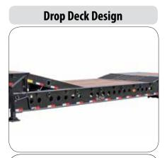
The drop deck design allows for taller loads.
